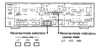
The reverse-mode selectors are used to select either of three different playback modes.
