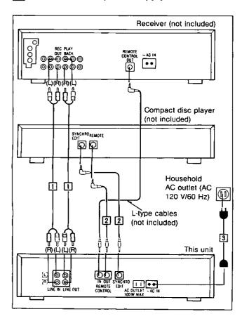
The illustration at the left shows an example of connections made when this unit is combined with a Technics hi-fi component system, and shows only the connections to be made to and from this unit in that combination.
